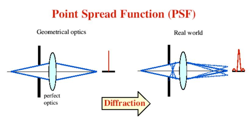
The PSF for a perfect optical system is the Airy disc, which is the Fraunhofer diffraction pattern for a circular pupil.
