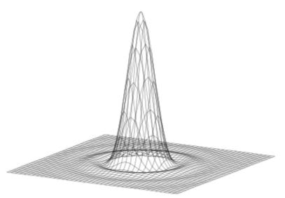
Every resolved object  $O(\alpha)$  can be considered as a composed by many point sources. Any point source generates its PSF. The image of the object  $I(\alpha)$  is given by the **convolution** of the object with the PSF.
