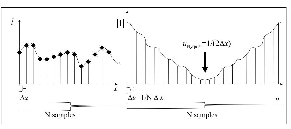
At least two samples per period for the highest frequency present in the signal.
